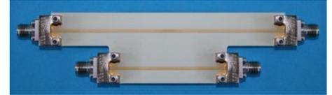
**1(b)** Extracts complex permittivity from directly measured S-parameters of a section of homogeneous transmission line (transmission coefficient egL) stored in Touchstone file using 3D EM line model. Multiline calkit and NIST Multiline TRL calibration technique is usually used for this option.
