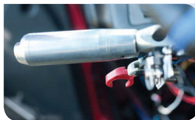
For their senior engineering project, Steven Georges (above), Joval Shamsoum (right), and Mike Carter (not pictured) designed a hand-operated clutch system for driving a manual transmission vehicle.
