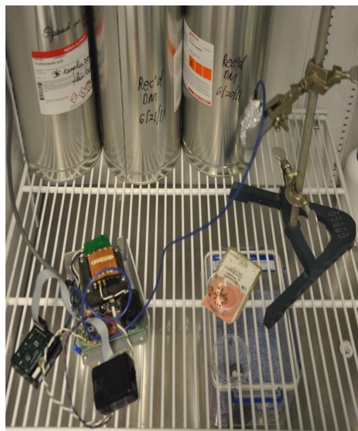
Figure 1: 830 nm laser in 4°C chromatography chamber.
