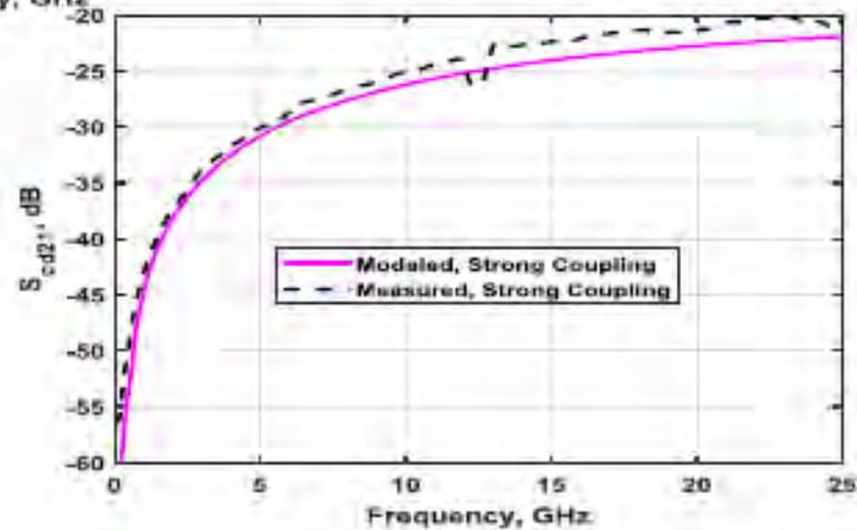
Line lengths are 80 mm and 80.254 mm (10 mil length imbalance)
