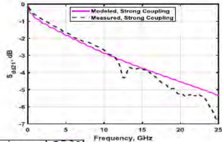
Modeled technological effects: dispersive PPO Blend, ERD, epoxy resin pocket, 60° trapezoid traces
