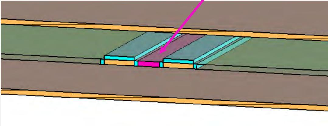
Epoxy pocket between traces. Strong coupled, rectangle edge, with ERD (surface roughness included)
