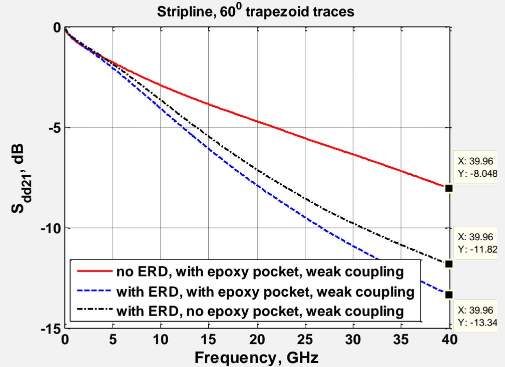
Comparing two ERD cases – with epoxy resin pockets and without, there is a difference of about 1.5 dB at 40 GHz for the given lengths of the traces in the IL for the DM propagation due to the epoxy pocket.
