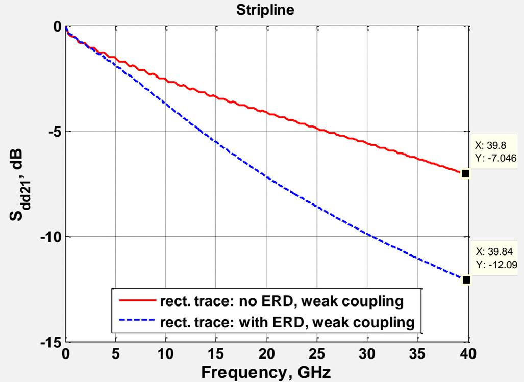
There is difference of about 5.0 dB at 40 GHz for the given lengths of the traces in the IL for the DM propagation.
