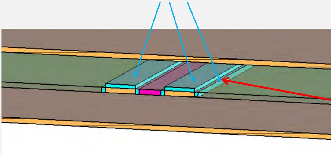
ERD (surface roughness). Strong coupled, rectangle edge, with epoxy pocket.
