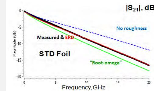
**Optimization procedure** uses numerical modeling in the loop for fitting S-parameters until measured and modeled results agree within some criteria.
