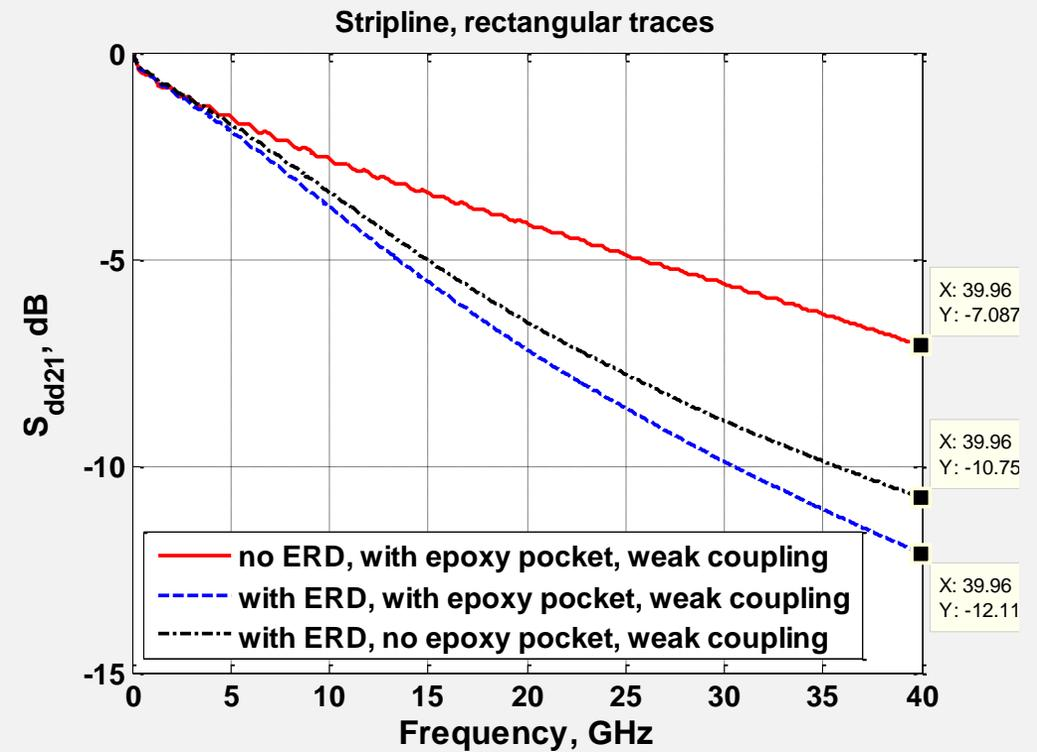
Comparing two ERD cases – with epoxy resin pockets and without, there is a difference of about 1.4 dB at 40 GHz for the given lengths of the traces in the IL for the DM propagation due to the epoxy pocket. This difference is less than for the strong-coupled case.
