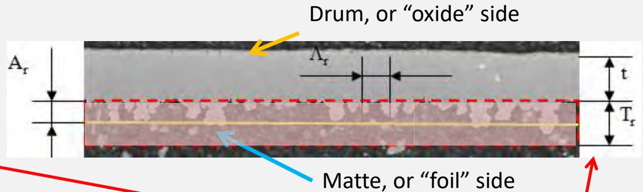
This inhomogeneous interface layer "copper-dielectric" is substituted by ERD
