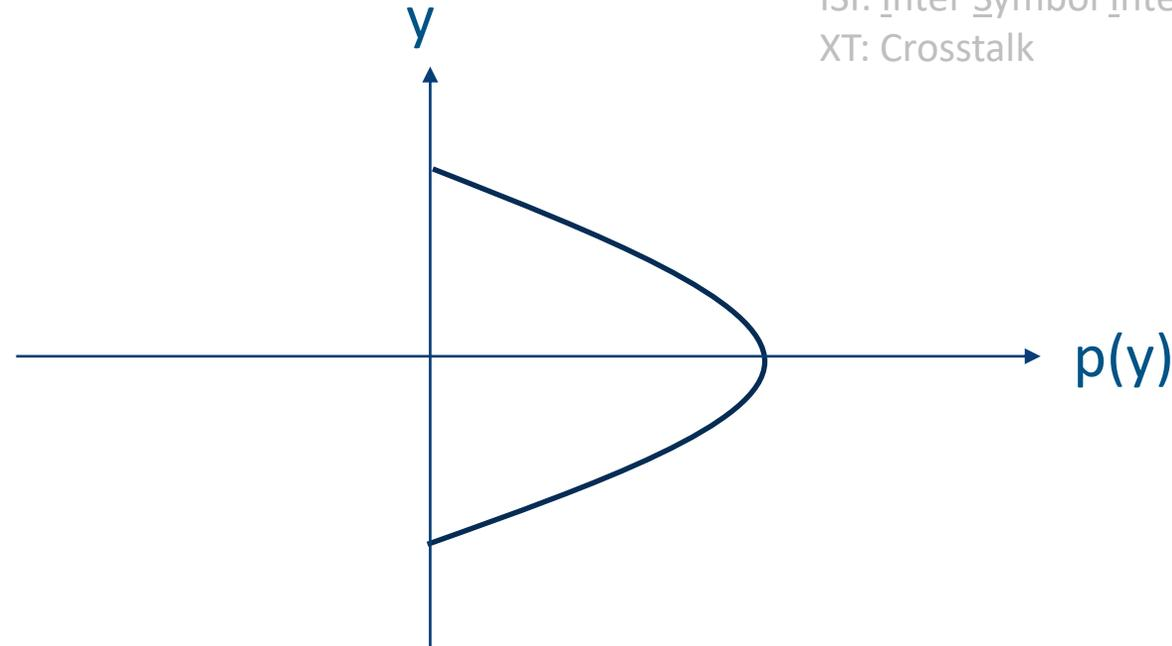
PDF  $p(y)$  is calculated by convolving DJ with RJ.
