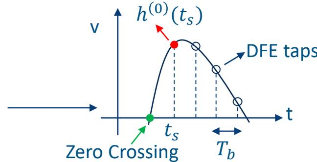
$h^{(0)}(t_s)$  : PR of THRU channel
