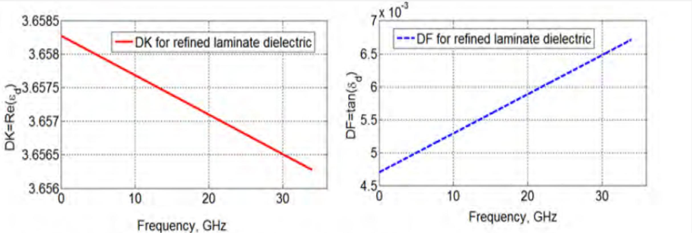
DK and DF of PPO Blend Dielectric extracted using DERM technique
